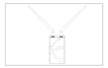
Position the antennas on transmitter and receiver as shown in the illustration. This ensures the best possible RF performance.
