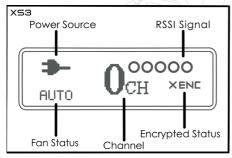
The RSSI display shows the strength of the signal, allowing the operator to check, if the system is working properly.
