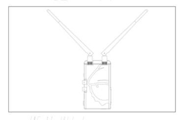
Position the antennas on transmitter and receiver as shown in the illustration. This ensures the best possible RF performance.
